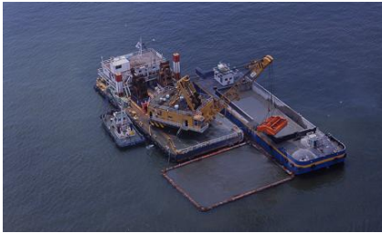
FIGURE 1. Conditions of waterway dredging by environmental dredging grab.
