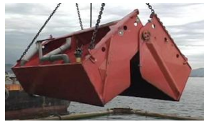
FIGURE 2. Shape of environmental dredging grab ( 7 \text{ m}^3 class).
